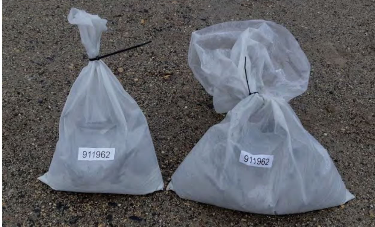
Figure 11-2: Principal RCGC Sample (Small) and Metallurgical Sample (Large) from a 2 m RCGC Interval
