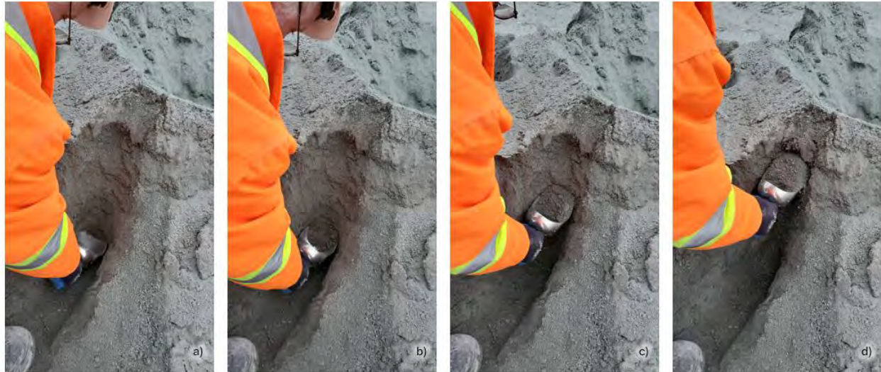
Figure 11-5: Full Bench Sampling on the “Short Wall” Face of the Spoil Pile
