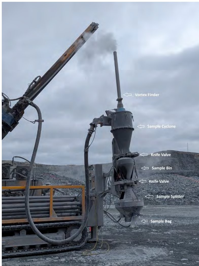
Figure 11-1: Hardab 5K6 Maxidrill RC Drill Rig with Metzke 1200 Cyclone w 3 Chute Cone Splitter (hyd) in Operation
