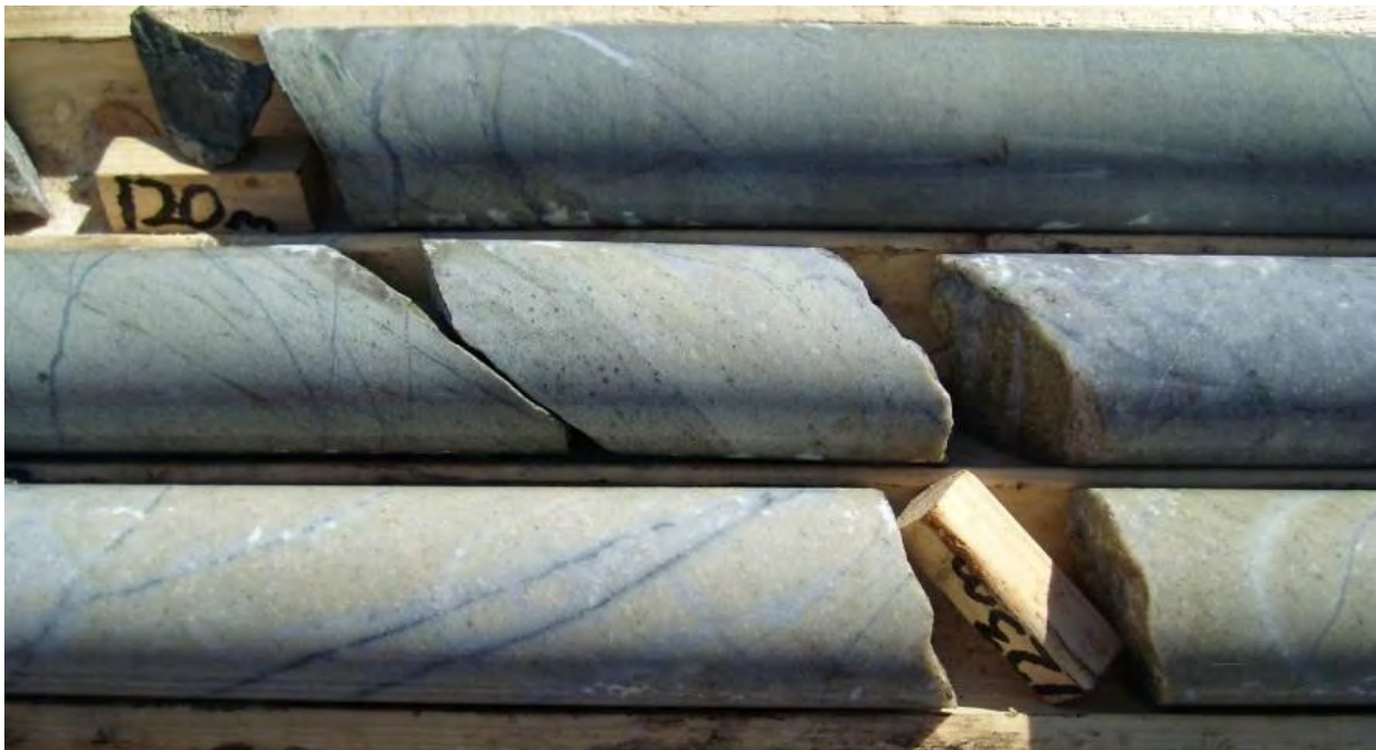
Figure 7-19: Example of Sericite-Altered Quartz-Feldspar Porphyry, 7.75 g/t Au
