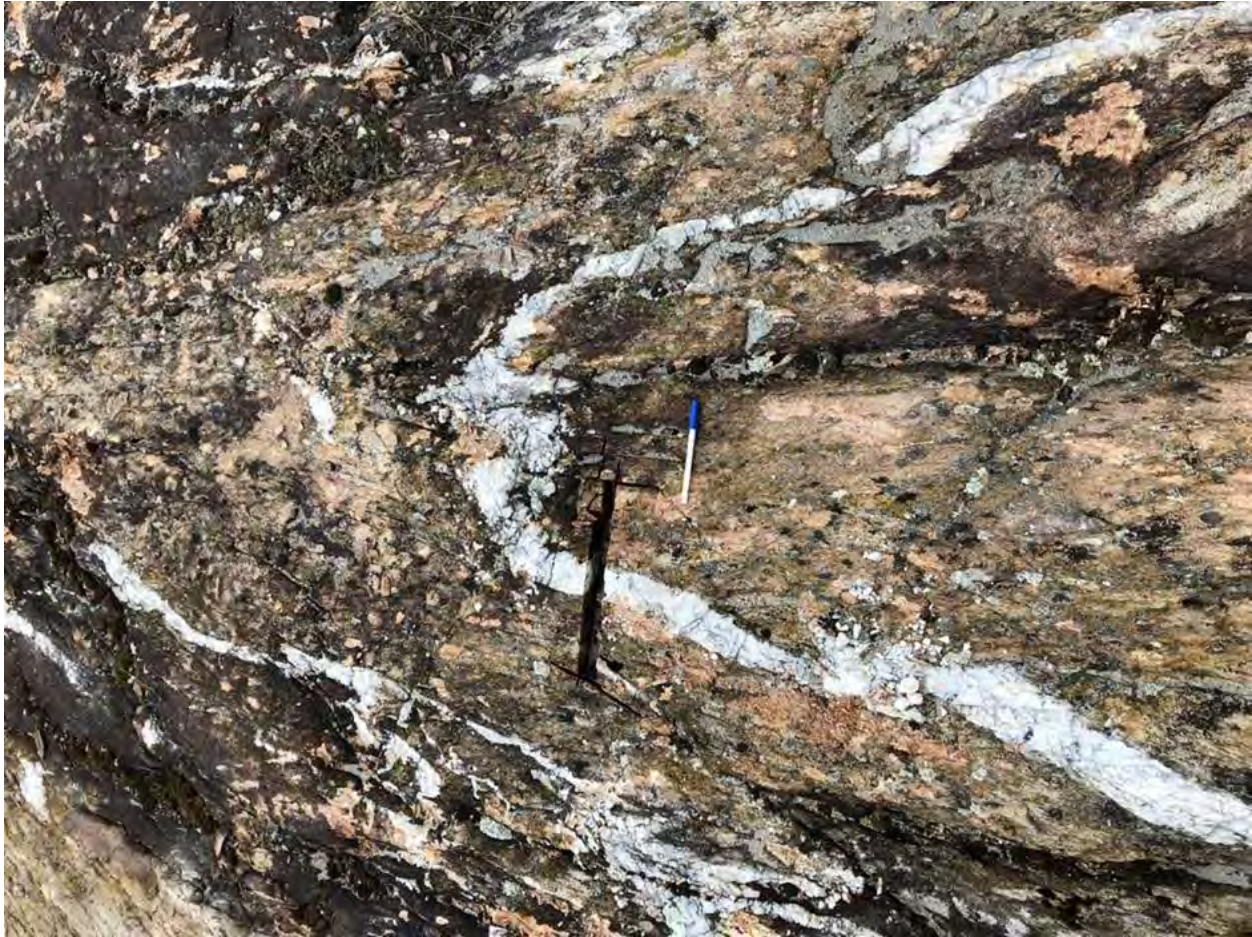
Figure 7-14: Folded Quartz-Carbonate Veins within Altered Quartz-Porphphyry, Porphyry Hill Sulphide Replacement Mineralization
