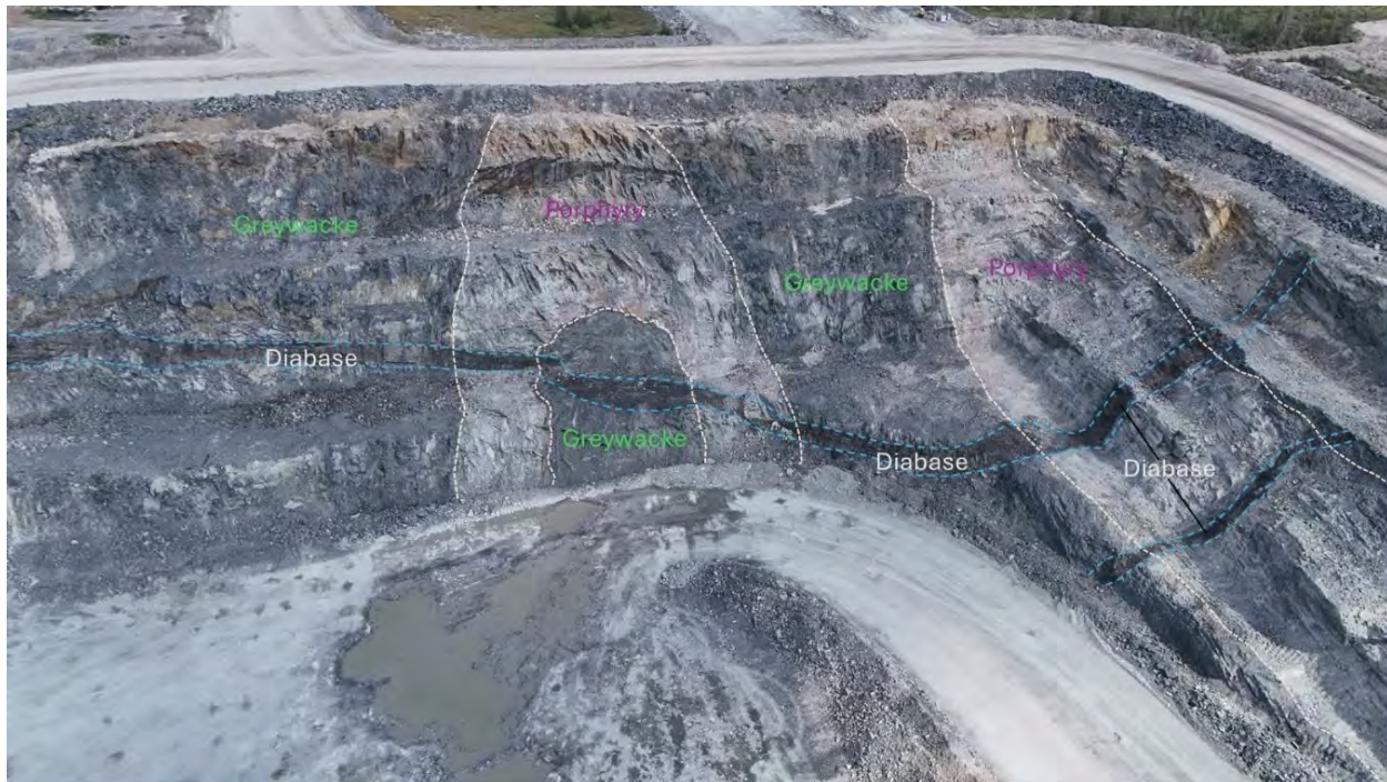
Figure 7-12: Greenstone Mine, East Pit at Southeast Corner—Folded Porphyry and Greywacke Units Crosscut by Younger Diabase Dykes
