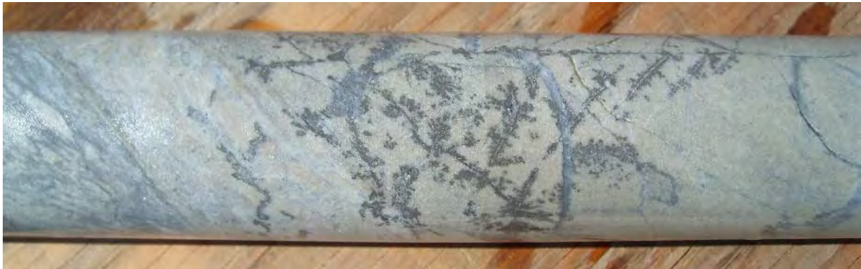
Figure 7-18: Example of Fracture-Controlled Pyrite Mineralization in Sericite-Silica Arkosic Wacke, 0.54 g/t Au
